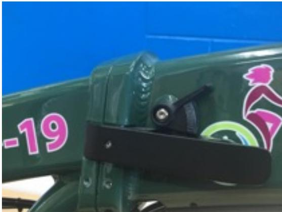
**Fig. 2: Safety latch in LOCK position**
