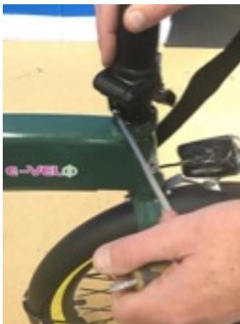
**Fig. 4a: Tighten side nut RHS**
