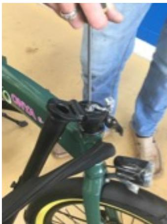
**Fig. 3: Tighten steering nut**
