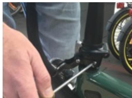
**Fig. 4b: Tighten side nut LHS**
